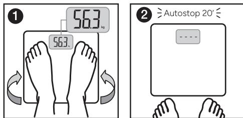
The measured weight flashes three times, then remains on the display for approx. 20 seconds.
